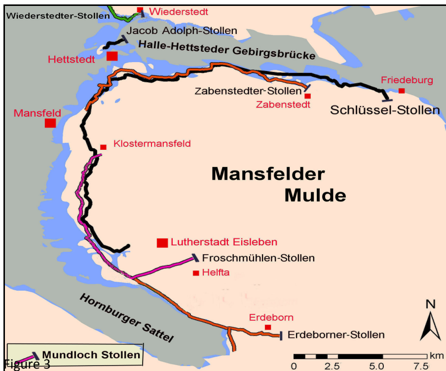
Figure 3 shows the localization of the most important still existing minewater drainage tunnels in the Mansfeld region.
